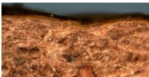
Fig. 9 - Leather for iPhone Case – papillary layer and finishing – detail
